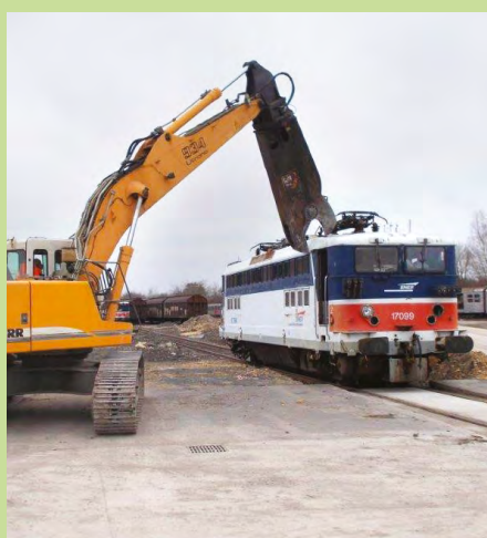
Breaking up a BB17099 electric locomotive ©All rights reserved
