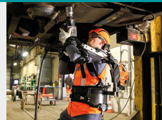
Shiva Exo is an exoskeleton developed with Ergosanté Technologie, shown here in the wagon workshop at our Nîmes-Courbessac Technicentre © Ergo Santé
