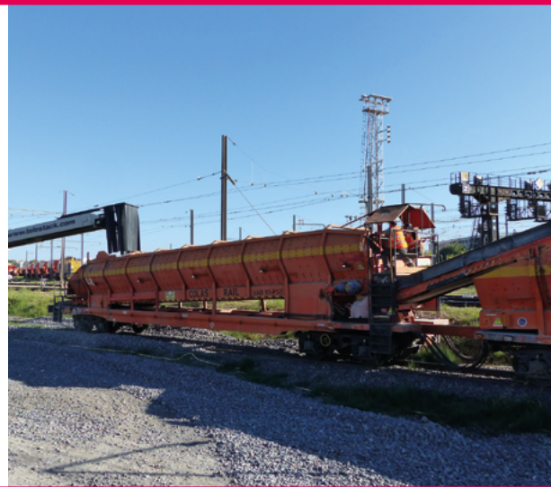
Recycling ballast at Cavaillon in southern France © Michel Lopez
