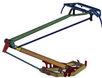
3D model of a pantograph for the study of pantograph/OCL interaction
