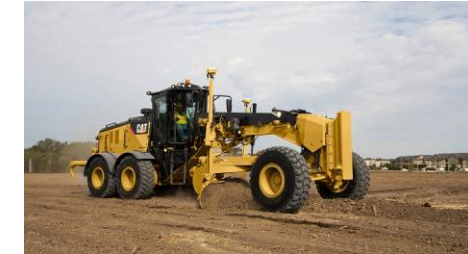
Figure 108 - Niveleuse (source: construction cayola)
